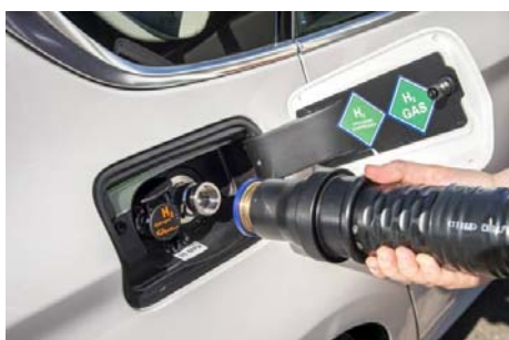
3 | Refuelling of hydrogen fuel tank © BMW Group | P90189152
