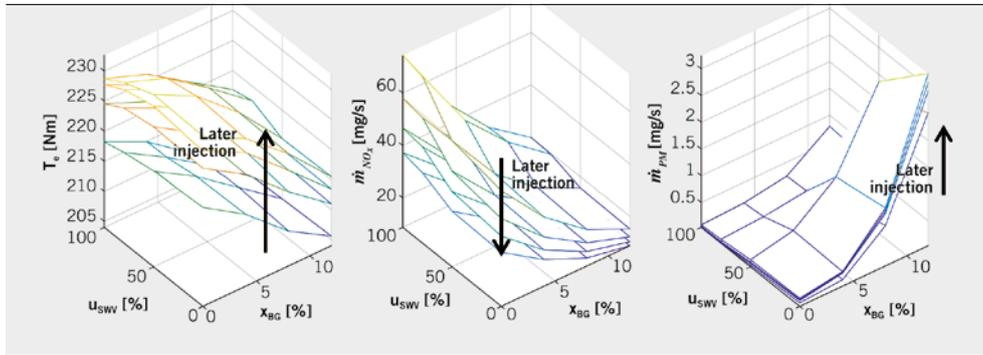
FIGURE 2 Engine response in terms of torque generation (left), nitrogen-oxide (middle) and soot emissions (right) at 1250 rpm and 40 % load (© ETH Zurich)
