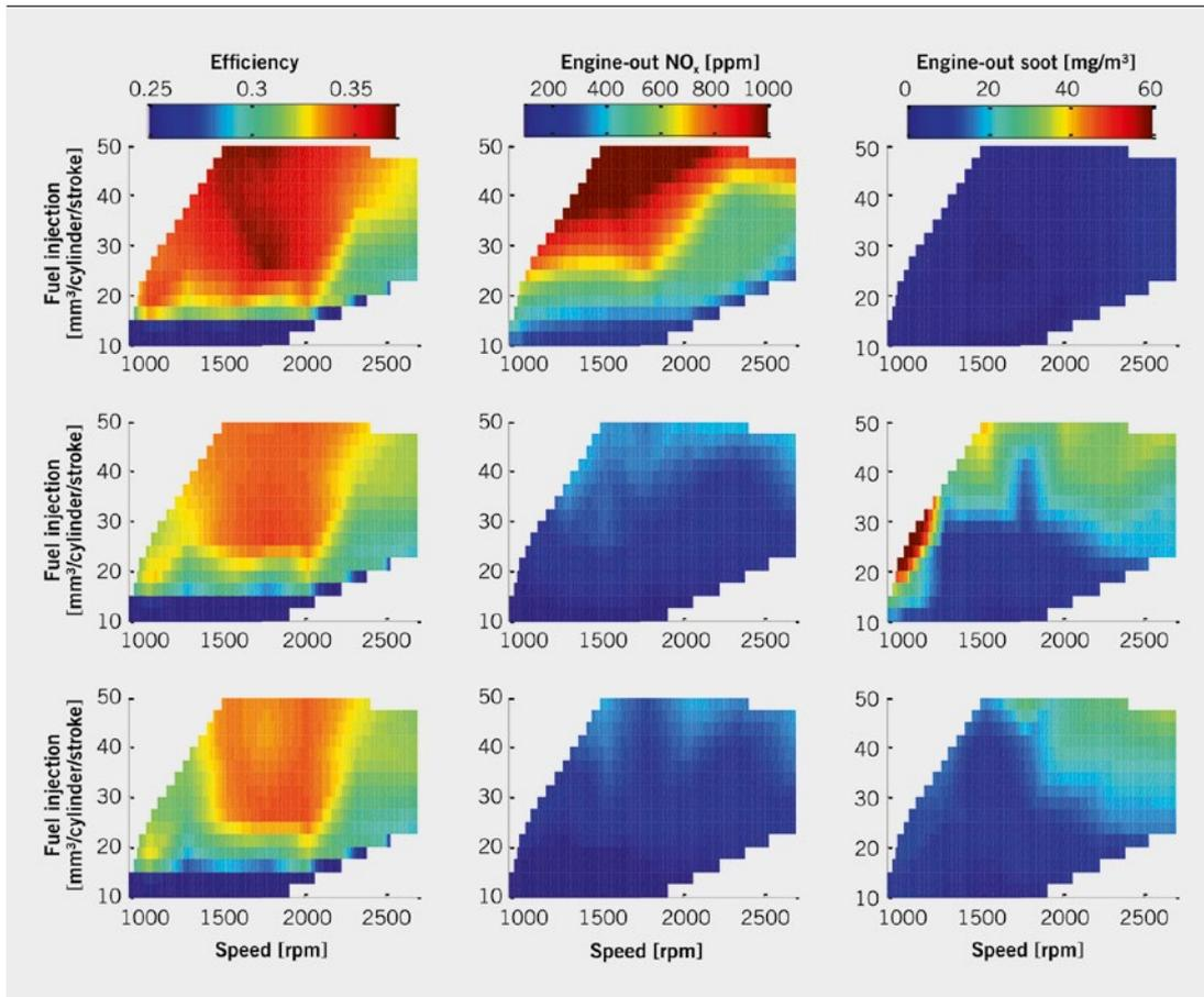
FIGURE 3 Efficiency, nitrogen oxide and soot emissions as a function of the operating point and the strategic value (top: fuel optimal, middle: low NO<sub>x</sub> without soot penalty, bottom: low NO<sub>x</sub> with soot penalty) (© ETH Zurich)
