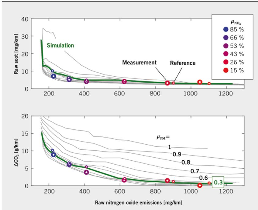
**FIGURE 5** Comparison of results from simulation and engine-in-the-loop experiment (the green curve represents the ideally achievable performance of the engine on the NEDC, the thick circles represent the cumulative values measured during the experimental test with six different emission strategies) (© ETH Zurich)
