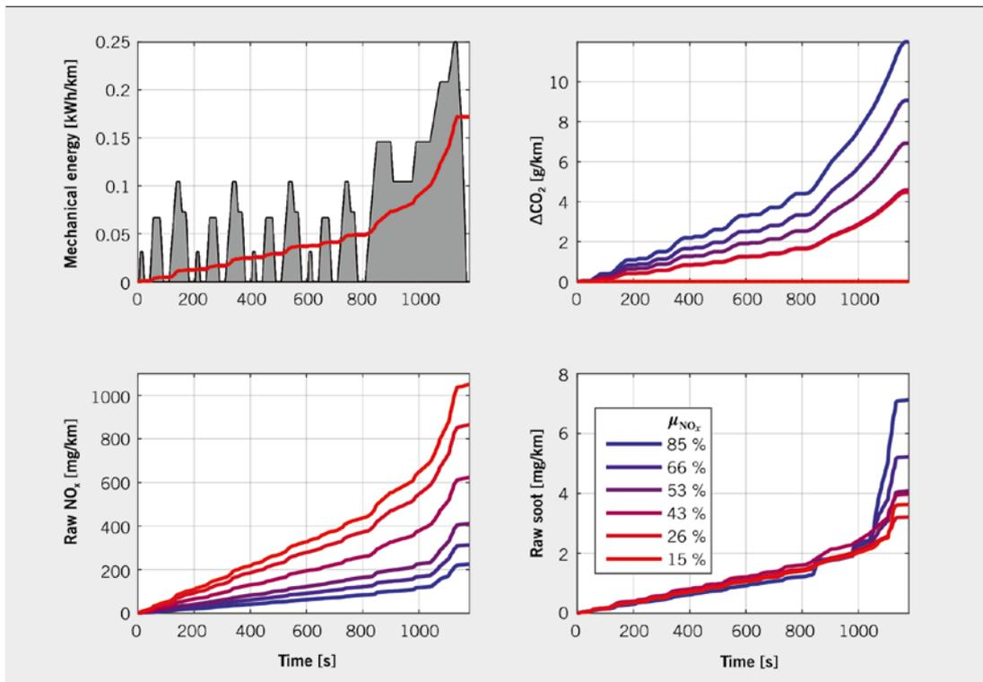
**FIGURE 4** Experimental test results of six different raw-emission strategies evaluated on the real engine using the NEDC (© ETH Zurich)
