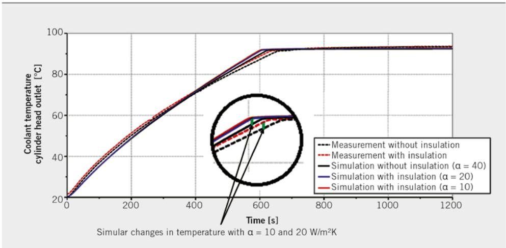
FIGURE 4 Temperature progression of the coolant for various heat transfer coefficients (© IMS)
