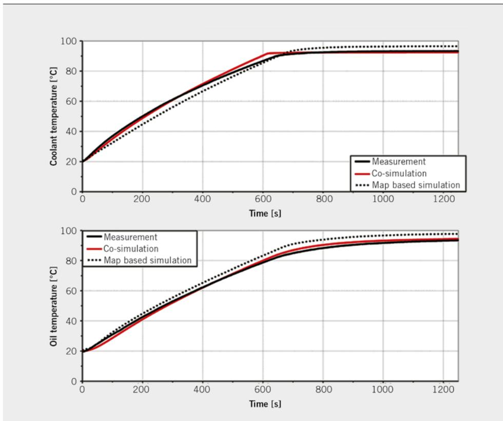
**FIGURE 1** Comparison of media temperatures (measured values and simulation) (© IMS)
