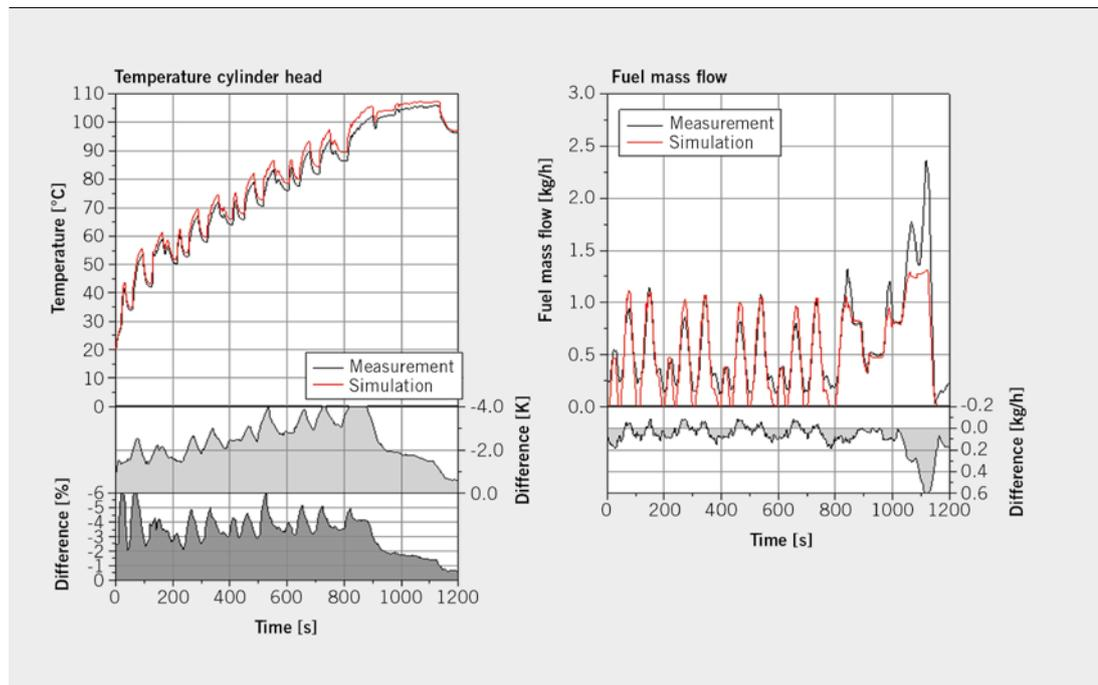
FIGURE 5 Temperature of the cylinder head (fire deck) and fuel mass flow (Ford 2.2 I in the NEDC) (© IMS)
