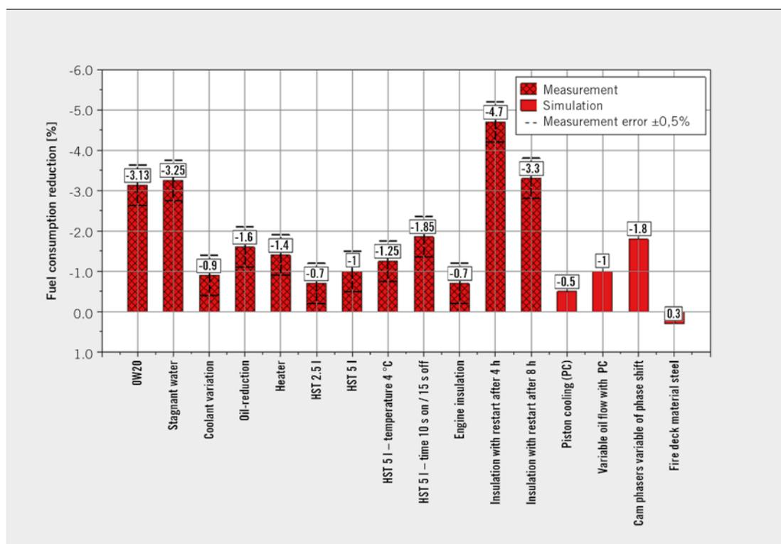
FIGURE 6 Comparison of all examined and simulated measures at 1500 rpm and 50 Nm (© IMS)
