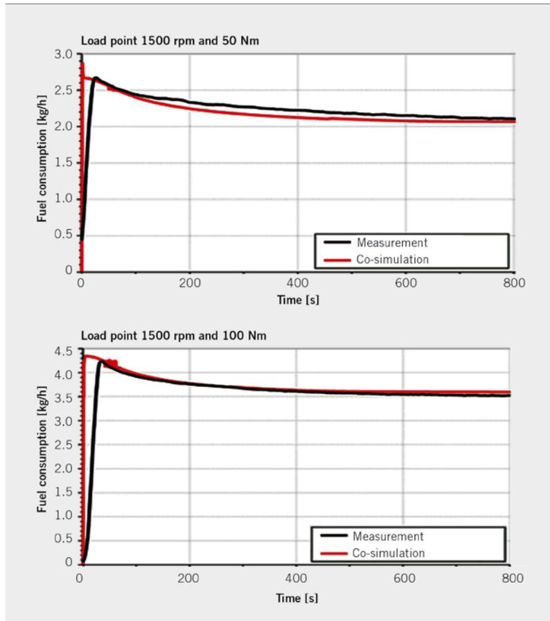
**FIGURE 2** Comparison of fuel mass flow (simulation and measured value) (© IMS)
