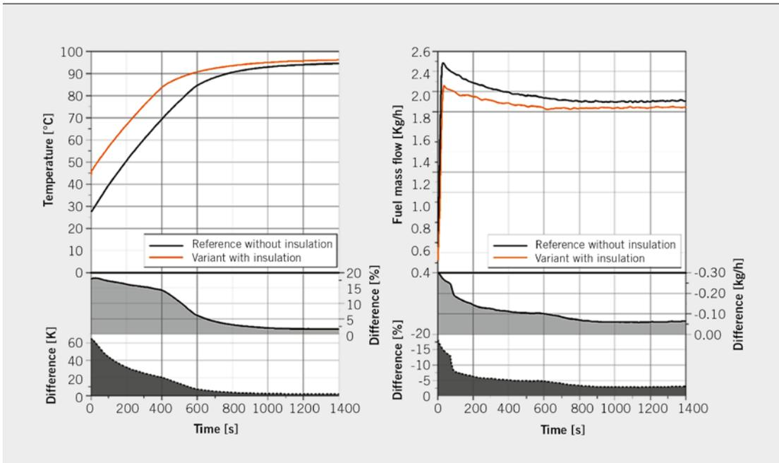
FIGURE 3 Oil temperature (left) and fuel mass flow (right) in comparison (load point 1500 rpm and 50 Nm) (© IMS)
