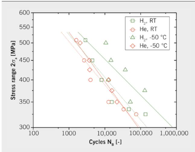
FIGURE 2 Fatigue tests (f = 1 Hz) (© University of Stuttgart)
