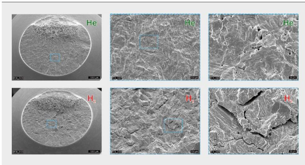
**FIGURE 6** Fractographic investigations (SEM) (© University of Stuttgart)
