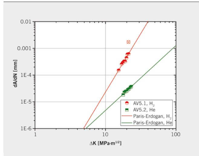
FIGURE 5 Crack growth curve (T = -50 °C) (© University of Stuttgart)
