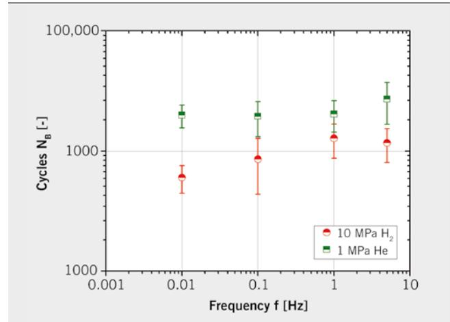
FIGURE 3 Influence of load frequency on the allowable number of load cycles (© University of Stuttgart)
