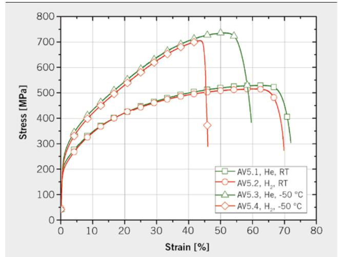
FIGURE 1 CERT tests (RT and T = -50 °C) (© University of Stuttgart)
