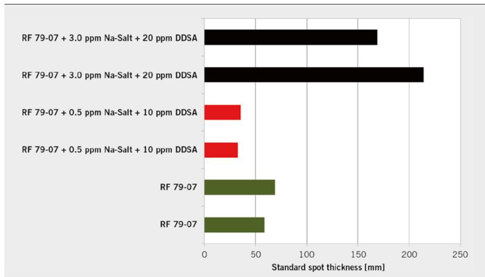
**FIGURE 8** Standard spot thickness of the deposits without and with the addition of soap formers to the reference DK 79-07 (© University of Rostock)
