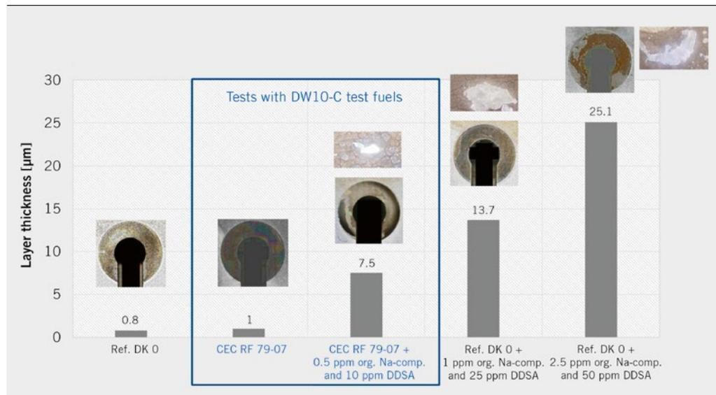
**FIGURE 10** Layer thicknesses on injector components (intermediate plates) after tests with DW10C reference fuels at the injection system test bench [11] (© University of Rostock)
