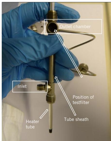
**FIGURE 4** Installation of heater tubes
