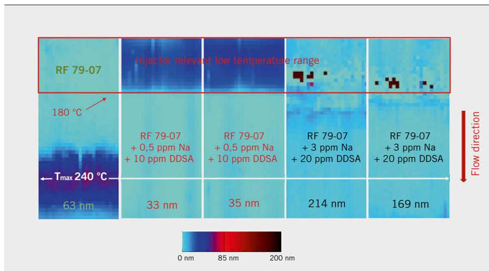
**FIGURE 9** Thickness maps of tubes with soap-like deposits (© University of Rostock)
