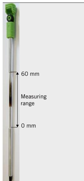
**FIGURE 3** Aluminum heater tube
