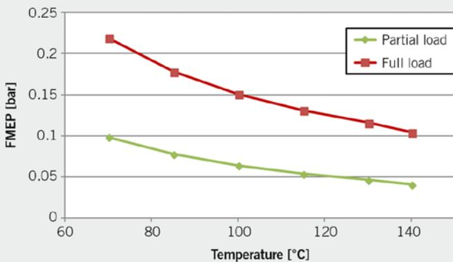
FIGURE 5 FMEP of the connecting rod bearings at  $n = 1500$  rpm (© iaf-mt)
