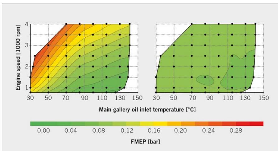
**FIGURE 1** Friction Mean Effective Pressure (FMEP) of the crankshaft (left) and of the valve train (right) in motored operation (© IVK)
