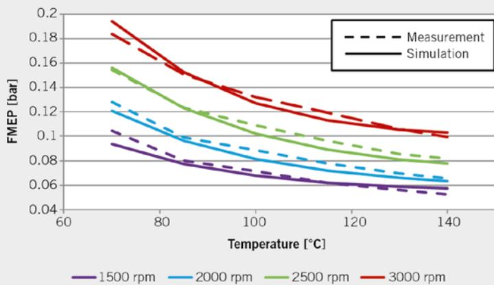
FIGURE 4 Motored friction of the main bearings in the crankshaft (© iaf-mt)
