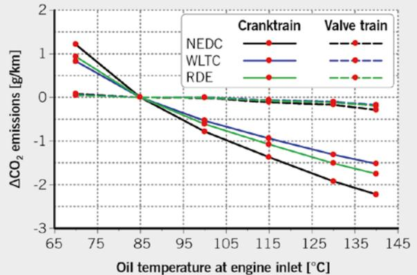
FIGURE 6 Changes of the  $\text{CO}_2$  emission for different driving profiles with variation of the oil temperature (reference temperature  $85^\circ\text{C}$ ) (© IVK)
