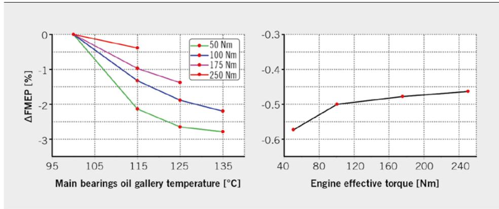
**FIGURE 2** Relative FMEP changes of the full engine at different loads (left) and due to oil temperature increase in the cylinder head from 90 to 110 °C (n = 2500 rpm) (© IVK)
