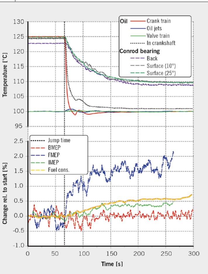
**FIGURE 3** Temperature behavior within the oil circuit of the main bearing at temperature jump ( $\Delta T = -10\text{ °C}$ ) and behavior of friction and combustion during the jump (Md = 54 Nm, n = 2500 rpm) (© IVK)
