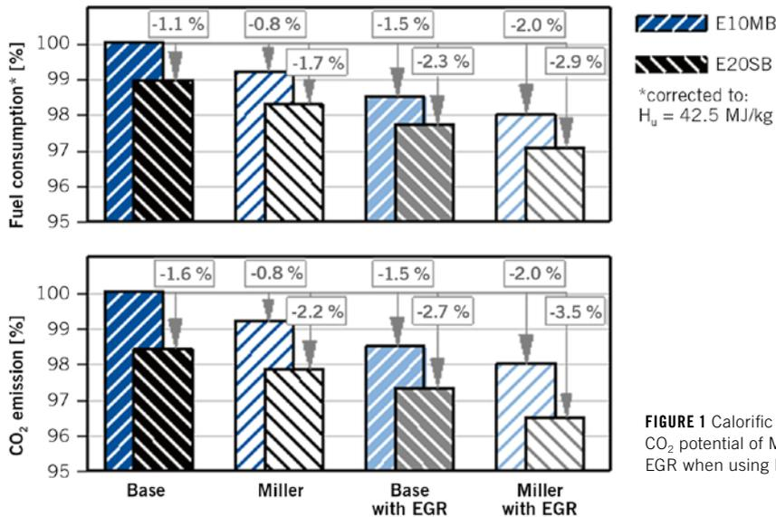
FIGURE 1 Calorific value-adjusted comparison of the CO<sub>2</sub> potential of Miller cycle and cooled external EGR when using E10 and E20 in NEDC (© VKA)
