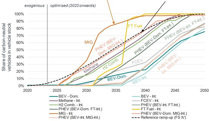
Reference Ramp-up FVV FS IV (just limited by vehicle fleet exchange rate, GHG neutrality in 2050)
