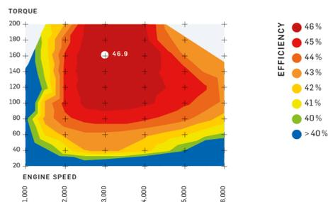
In methanol operation, the new ultimate efficiency engine achieves an efficiency of at least 40% over almost the entire engine characteristic map.
