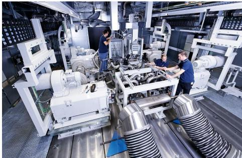
The results from vehicle and engine simulation as well as the influence of carbon-neutral fuels on engine behaviour are tested on a single-cylinder research engine.
