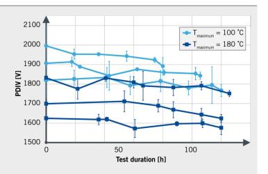
FIGURE 3 Degradation tests for different maximum temperatures (© IMA)
