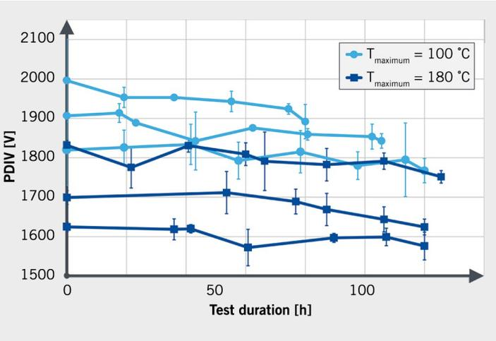
**FIGURE 3** Degradation tests for different maximum temperatures (© IMA)
