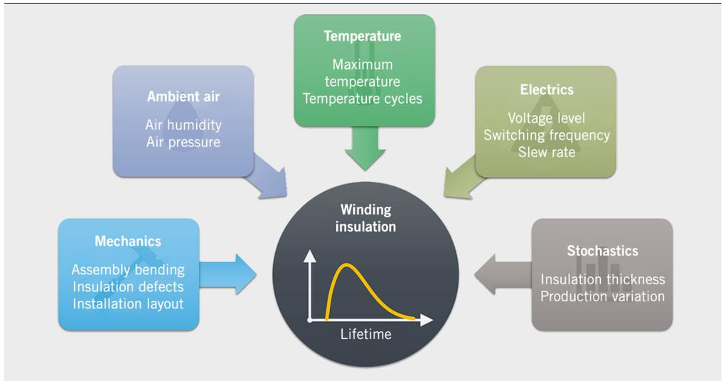
**FIGURE 2** Categorized potential influencing parameters for the degradation and the lifetime of the winding insulation (© IMA)
