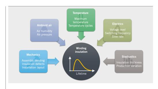
FIGURE 2 Categorized potential influencing parameters for the degradation and the lifetime of the winding insulation (© IMA)
