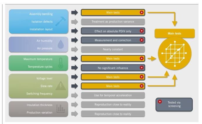
FIGURE 4 Treatment of the previously categorized potential influencing variables and assignment to screening tests or main tests (© IMA)
