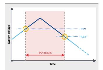
FIGURE 1 Schematic representation of the occurrence of PD (© IMA)
