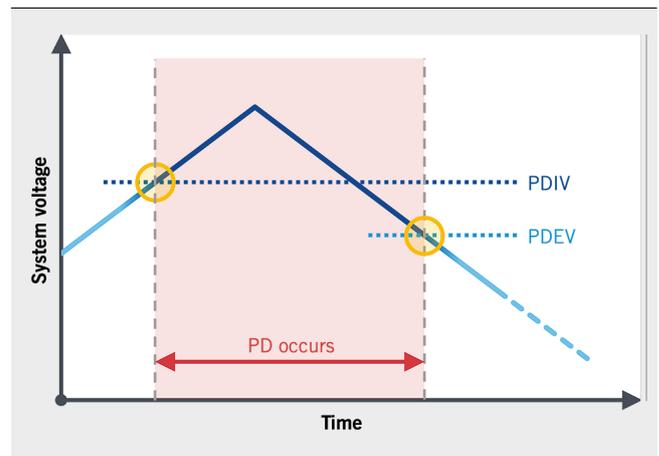
**FIGURE 1** Schematic representation of the occurrence of PD (© IMA)
