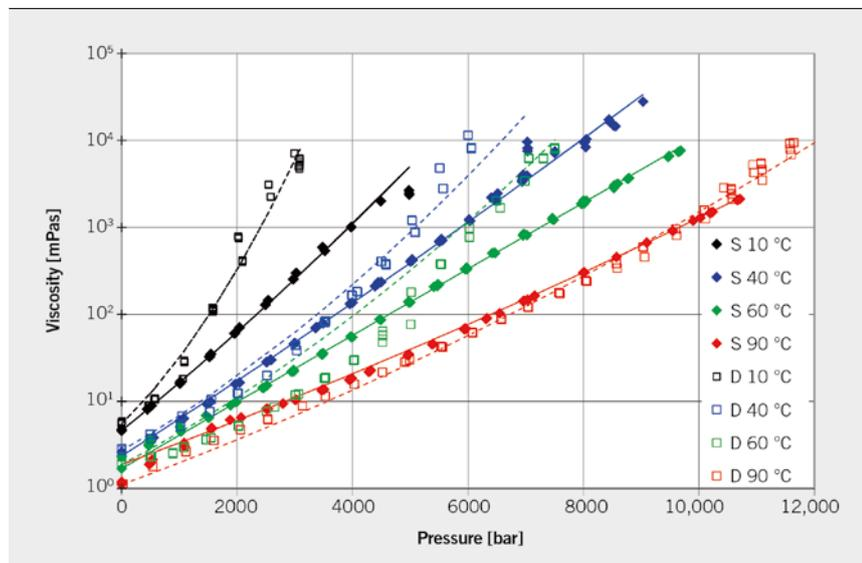
FIGURE 3 Dependence of the viscosity on the pressure and temperature for two diesel fuels (© ITR)
