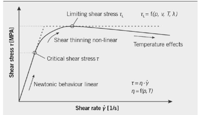
**FIGURE 1** Dependence of the shear stress on the flow behaviour of a fluid (© ITR)
