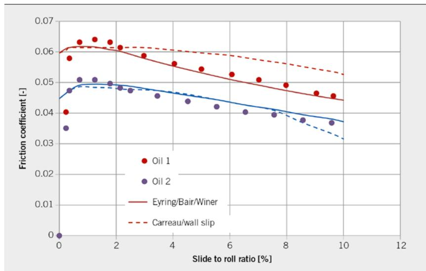
FIGURE 4 Comparison between experiment and simulation (traction curves at 60 °C, 10 m/s, 1420 MPa) (© ITR)
