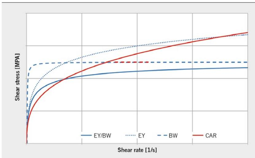
**FIGURE 2** Flow models (characteristic curves) (© ITR)
