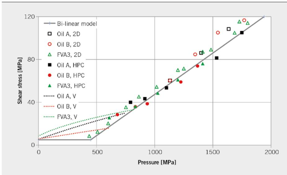
FIGURE 5 Dependence of the limiting shear stress on the pressure (© ITR)
