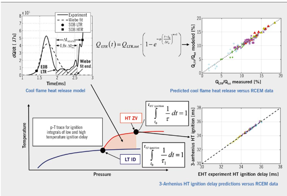
**FIGURE 5** Combination of 3-Arrhenius model and the developed model for cool-flame heat release (upper row) with two Livengood-Wu ignition integrals for low- and high-temperature ignition; integration along the pressure/temperature evolution during the compression stroke (lower left) allows for excellent prediction of main ignition onset (lower right) (colours correspond to fuels in **FIGURE 1**) (© LAV)
