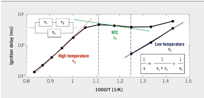
**FIGURE 4** Ignition delays times for fuels exhibiting two-stage ignition behaviour with characteristic low-, intermediate (NTC) and high-temperature regimes and corresponding 3-Arrhenius model (© LAV)
