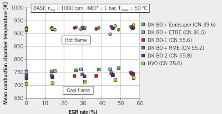
**FIGURE 3** Average combustion chamber temperature at start of cool-flame and high temperature ignition for a variation in EGR rate at one operating condition in the BASF engine (© IVK)
