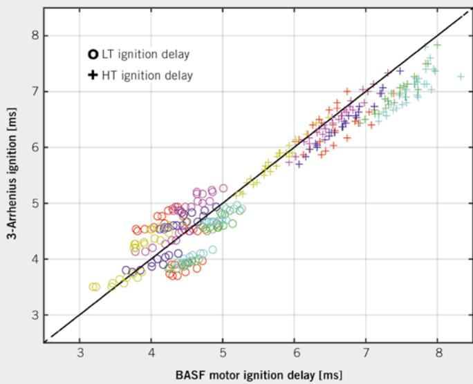
**FIGURE 6** Comparison between predicted and measured low and high temperature ignition delays when applying the surrogate fuel parameterisation from the RCEM to the OM642 engine running on the original fuels (colours correspond to fuels in **FIGURE 1**) © IVK and LAV
