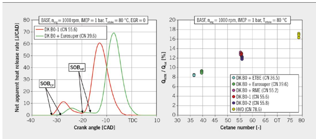
**FIGURE 2** Comparison of heat release rates for HCCI combustion of two different CN fuels in the BASF engine (left) and arrows indicate start of burn of cool-flame and high temperature ignition; ratio of cool-flame to total heat release as a function of CN for all fuels (right) (© IVK)
