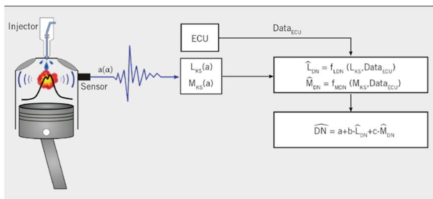
FIGURE 3 Methods for determining diesel noise rating (© IMS)
