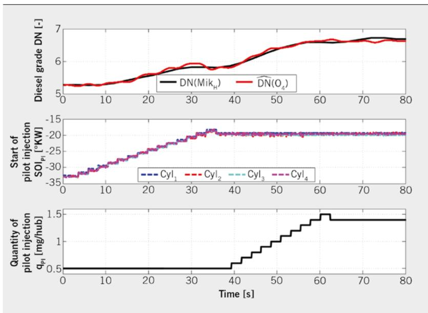
FIGURE 6 Development of the diesel noise rating (DN) and pilot injection parameter over time on running the optimisation algorithm (© IMS)
