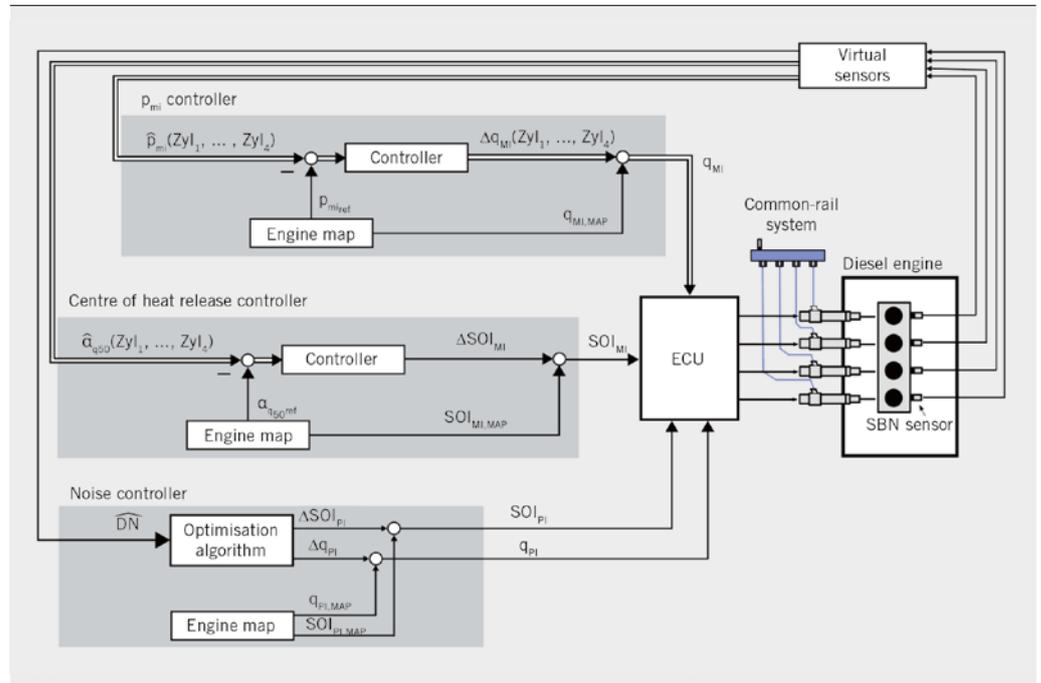
**FIGURE 4** Diagram illustrating the principle behind the control structure (© IMS)
