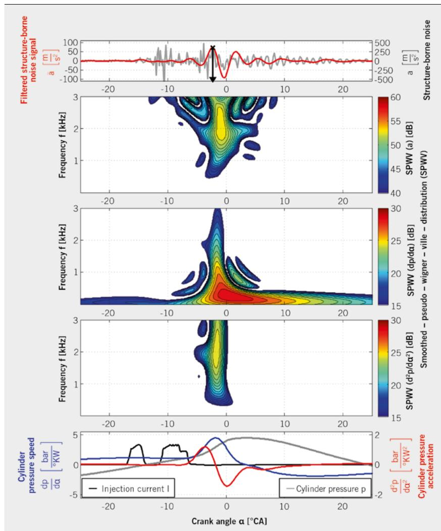
FIGURE 2 Time-frequency analysis of structure-borne noise signal a of sensor O<sub>1</sub> in comparison to cylinder pressure p of the first cylinder, cylinder pressure speed dp/dα and cylinder pressure acceleration d<sup>2</sup>p/dα<sup>2</sup> (1250 rpm, 25 Nm) (© IMS)
