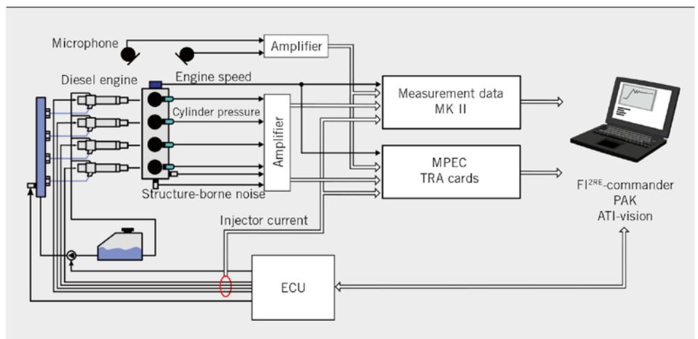
**FIGURE 1** Schematic diagram of test bench configuration
