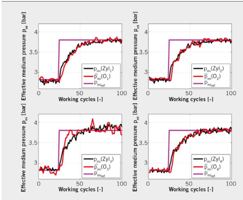
FIGURE 5 Step response of  $p_{mi}$  control to positive setpoint, plotted as a function of the working cycles (WC); the diagrams show the reference value, the measured and estimated  $p_{mi}$  value in relation to the individual cylinders and structure-borne noise sensors (© IMS)
