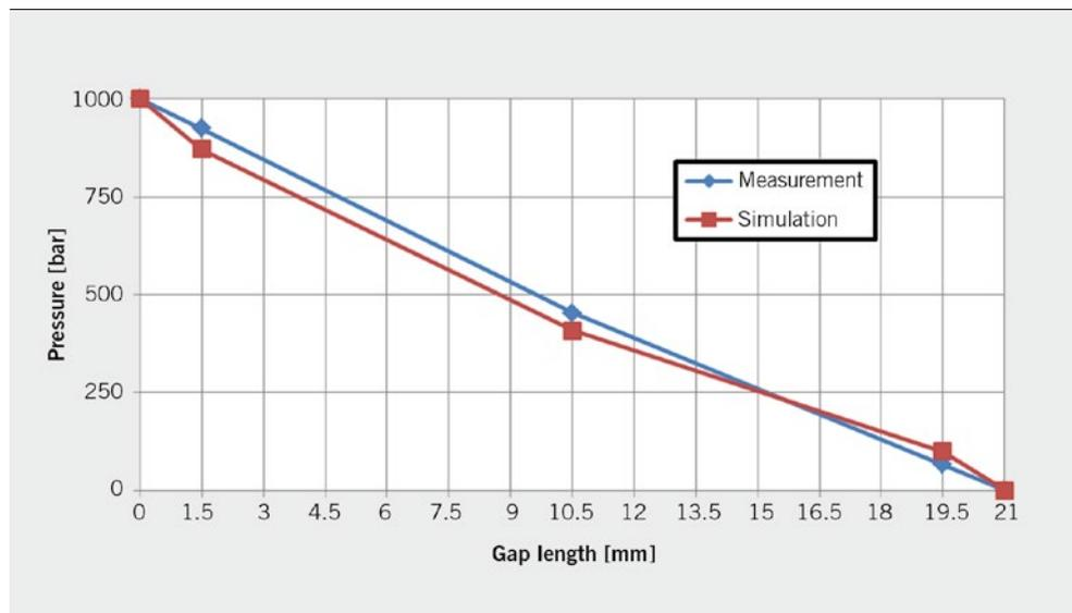
FIGURE 2 Pressure distribution over the gap length (© University of Kassel)
