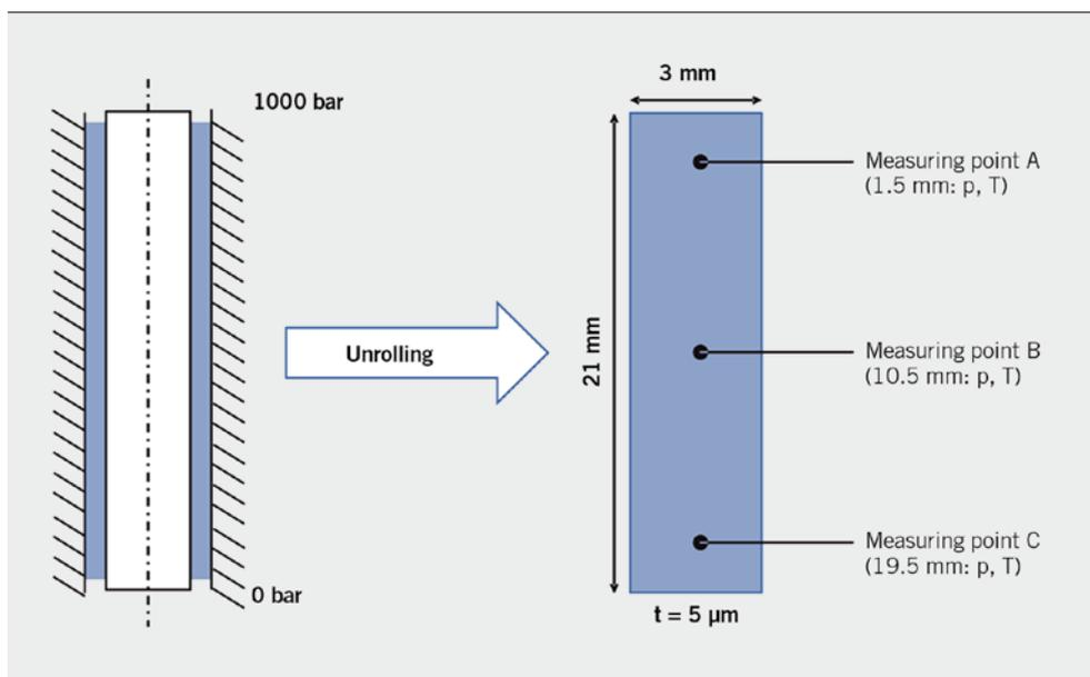
**FIGURE 1** Functional principle of the flat gap with measurement positions along the gap (© University of Kassel)
