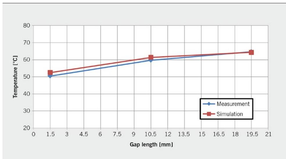
FIGURE 3 Temperature distribution over the gap length (© University of Kassel)
