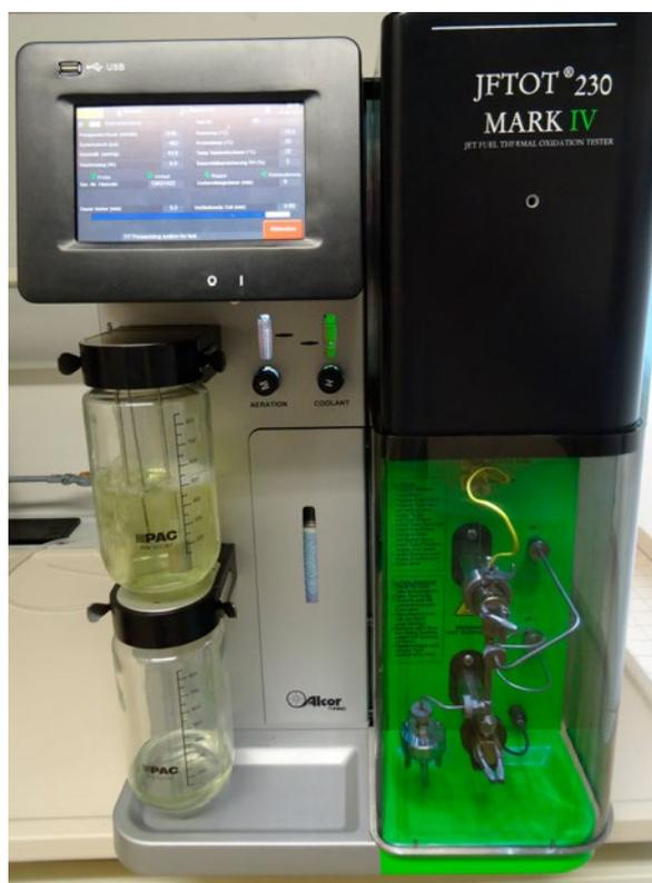
**FIGURE 2** Laboratory setup for the Diesel Deposit Formation Test (DDFT) © LVK Rostock)
