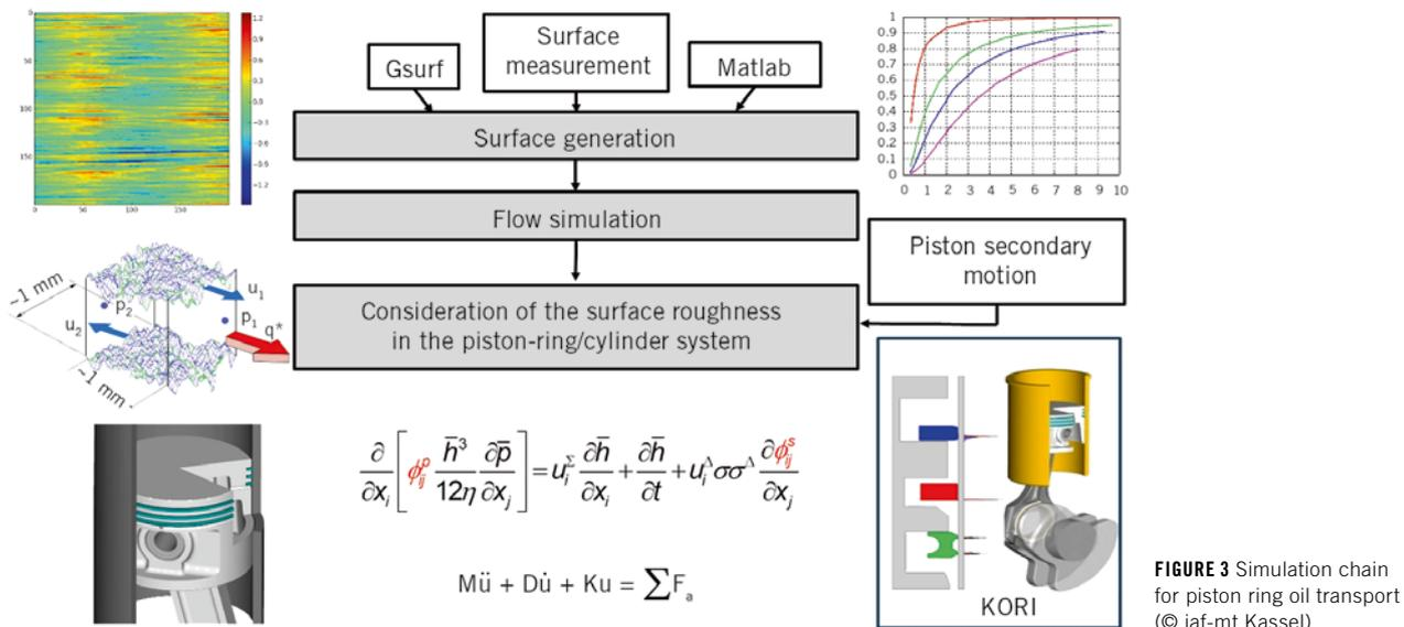
FIGURE 3 Simulation chain for piston ring oil transport (© iaf-mt Kassel)
