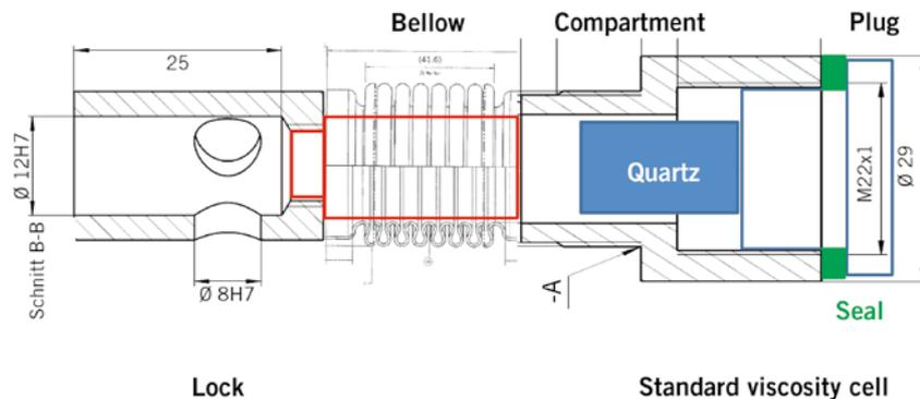
FIGURE 1 Test bench concept for shock-pressure measurements (© ITR Clausthal)
