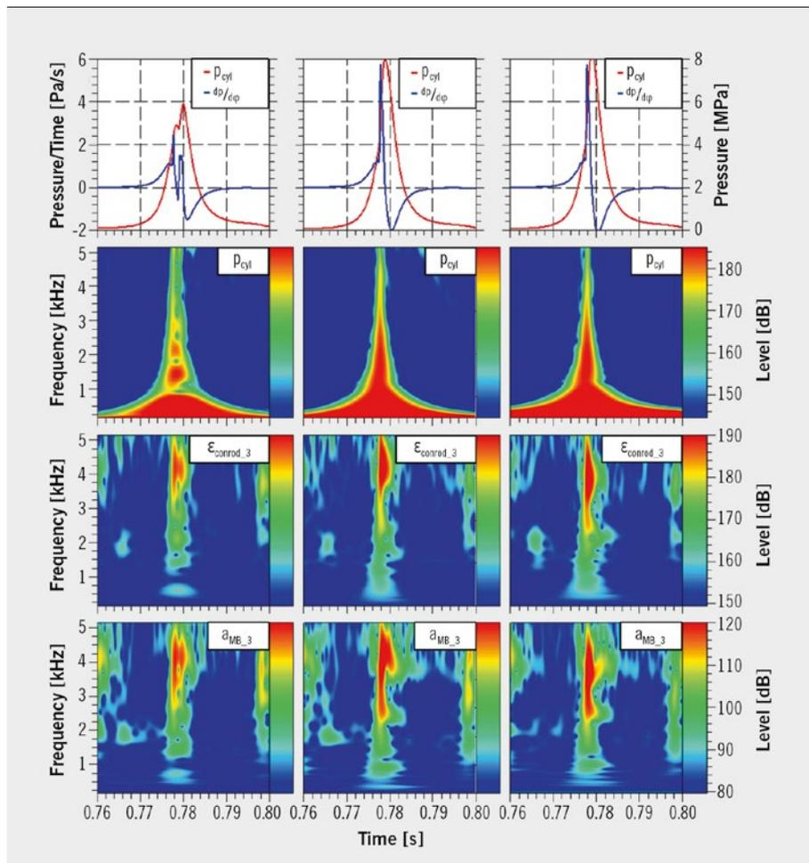
FIGURE 3 Wavelet analysis of cylinder pressure ( $p_{cyl}$ ), conrod elongation (second derivate of time ( $\epsilon_{conrod_3}$ ), and acceleration at main bearing in stroke direction ( $a_{MB_3}$ ) at 1500 rpm and 7.2 bar indicated mean effective pressure (left: serial conrod and pressure gradient, middle: serial conrod and maximum pressure gradient; right: weakened conrod and maximum pressure gradient) © University of Stuttgart
