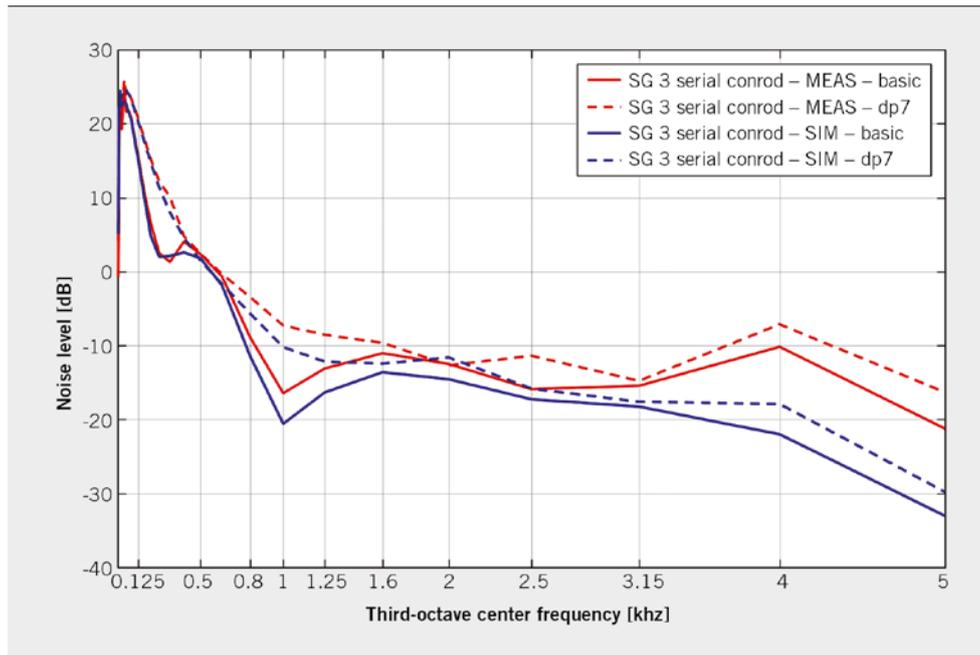
**FIGURE 5** Comparison of measurement and simulation for two different combustion excitations and serial conrod (© University of Stuttgart)
