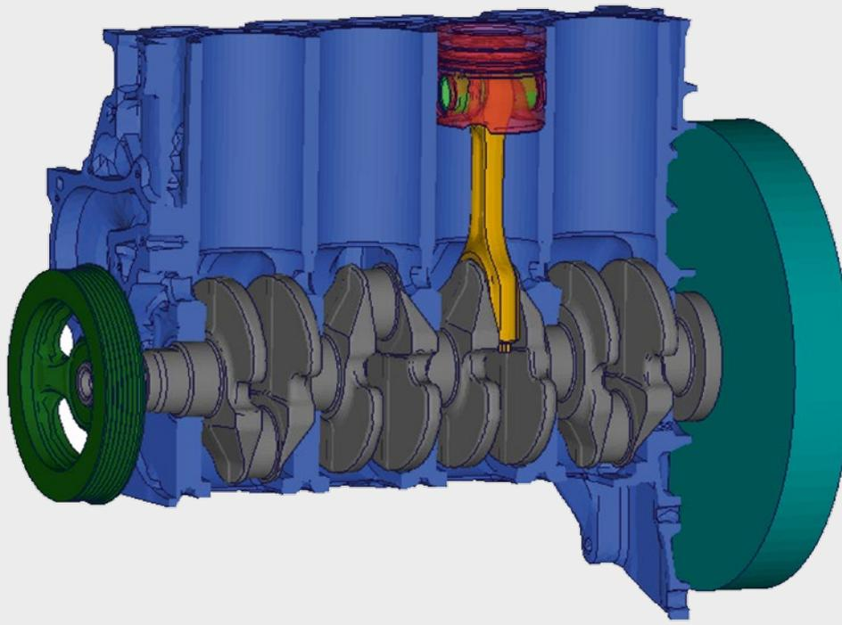
**FIGURE 4** Simulation model of the 1.5-l Euro 6 diesel engine (© University of Kassel)
