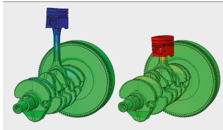
**FIGURE 2** FEA result of the longitudinal natural vibration of the conrod in assembled conditions (© University of Kassel)
