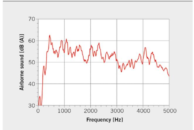
**FIGURE 1** Airborne sound at 1 m distance on cold engine side (© University of Stuttgart)
