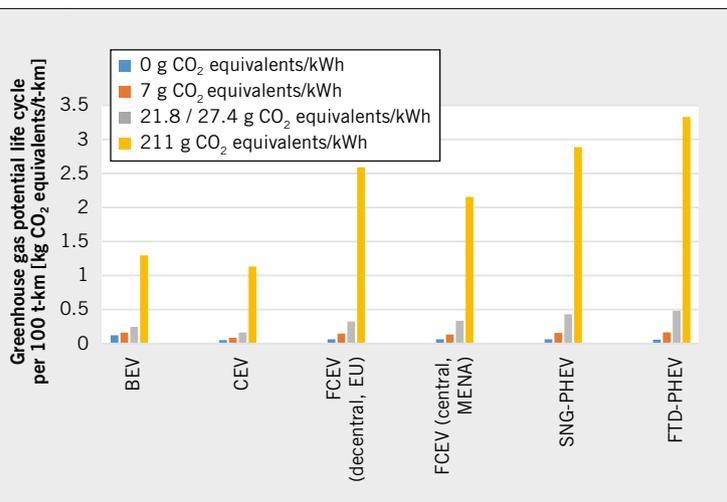
**FIGURE 4** Greenhouse gas potential over the life cycle for different energy scenarios (© University of Stuttgart, Institute for Acoustics and Building Physics)
