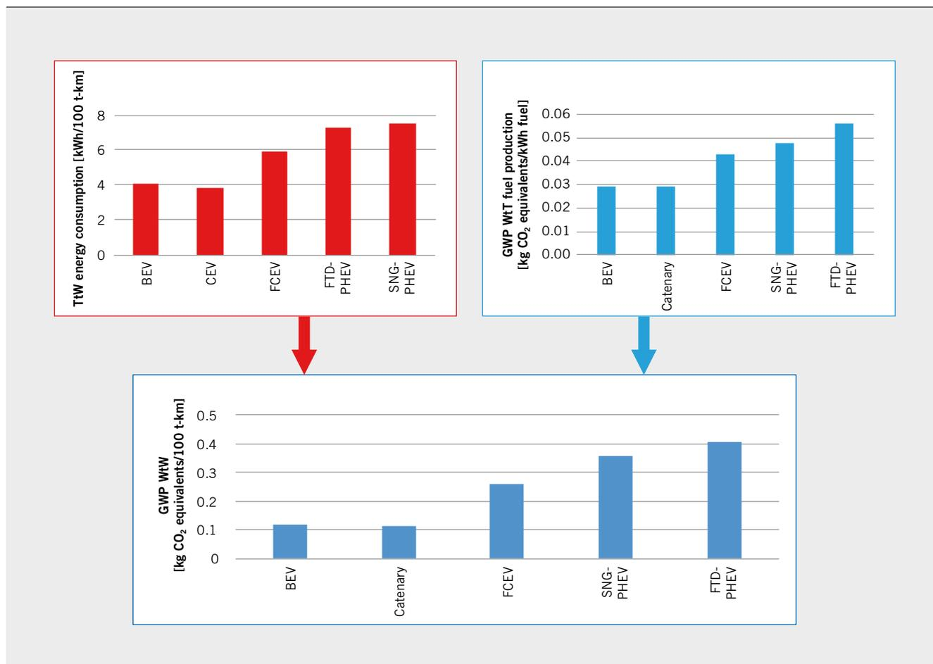
FIGURE 2 Greenhouse gas well-to-wheel evaluation (© University of Stuttgart, Institute for Acoustics and Building Physics)
