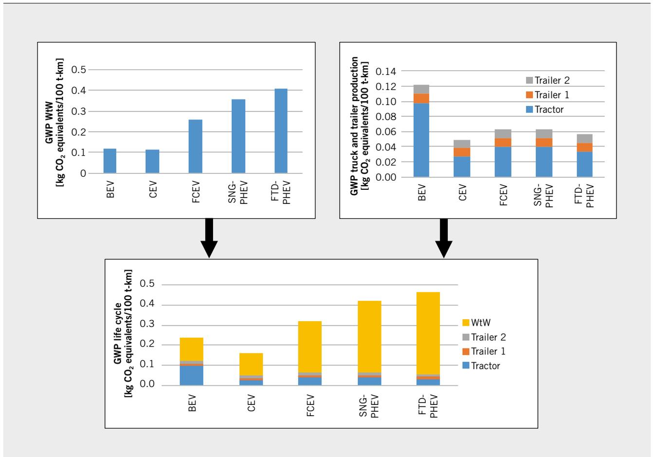
**FIGURE 3** Greenhouse gas potential for the whole life cycle (© University of Stuttgart, Institute for Acoustics and Building Physics)
