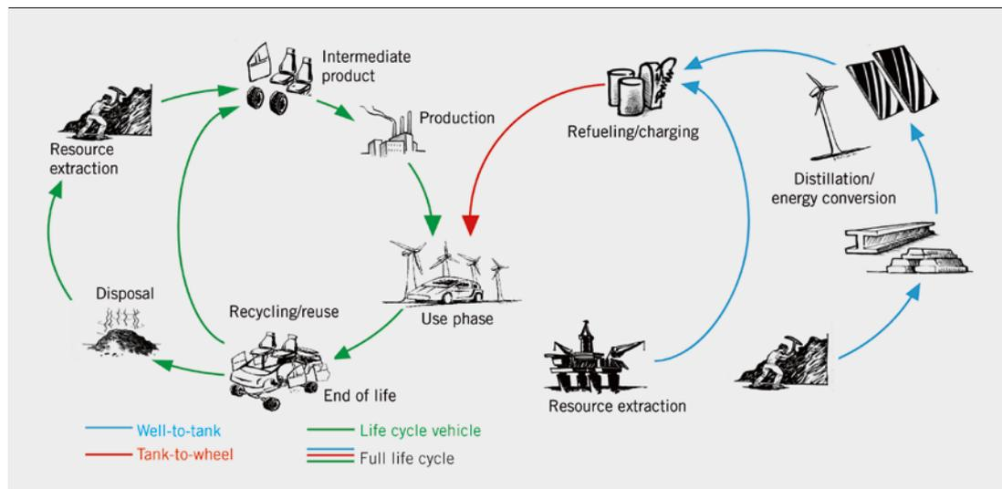
FIGURE 1 Overview well-to-wheel and full life cycle [4] (modified) © University of Stuttgart | Fraunhofer IBP
