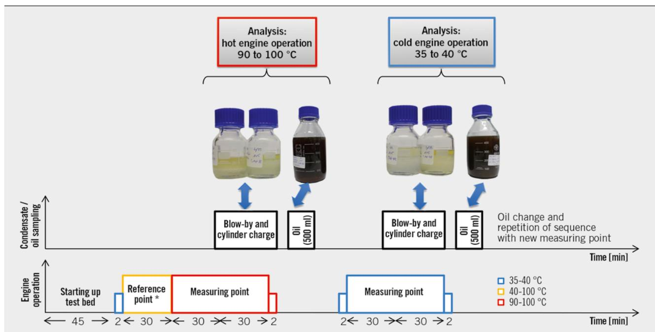
FIGURE 3 Flow chart of sample extraction of blow-by gas and cylinder gas (© LKV)
