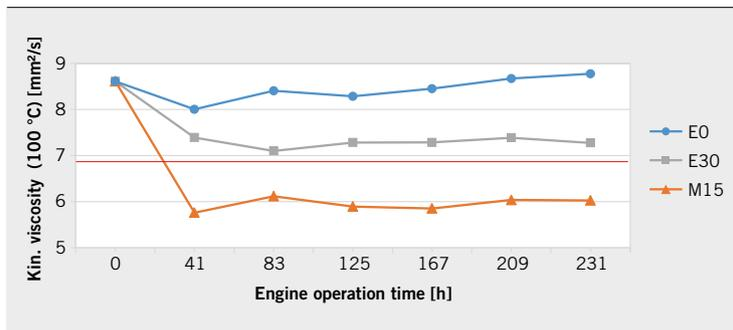
**FIGURE 4** Chart of the kinematic viscosity of the lubricating oil at 100 °C over the engine long-term tests (© LKV)
