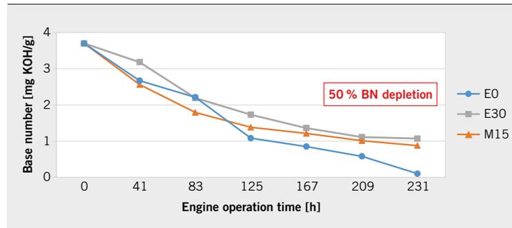
**FIGURE 5** Chart of lubricating oil base number over the engine long-term tests (© LKV)
