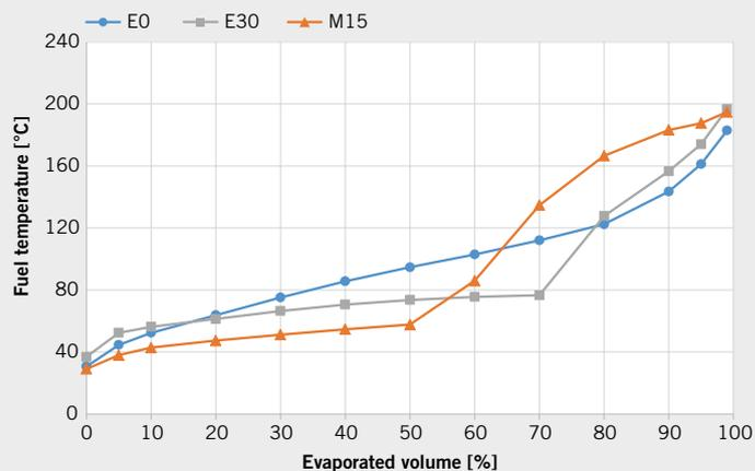
FIGURE 2 Boiling characteristics of test fuels (© LKV)
