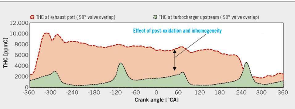
**FIGURE 1** Measured concentration of unburned hydrocarbons (Total Hydrocarbons, THC) in the outlet duct and downstream of the turbocharger for an operating point at 1600 rpm, at medium load and 90° valve overlap (© FVV)
