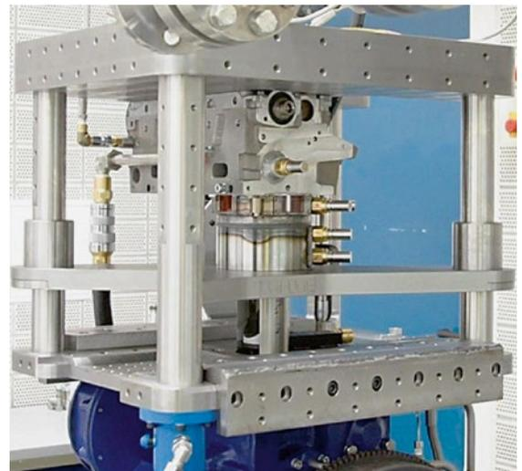
**FIGURE 5** Optically accessible diesel engine of the University of Duisburg-Essen in Germany (© University of Duisburg-Essen)
