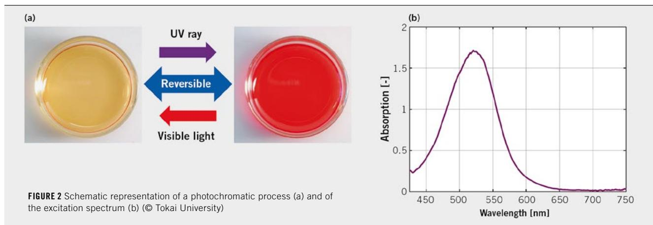
**FIGURE 2** Schematic representation of a photochromatic process (a) and of the excitation spectrum (b) (© Tokai University)
