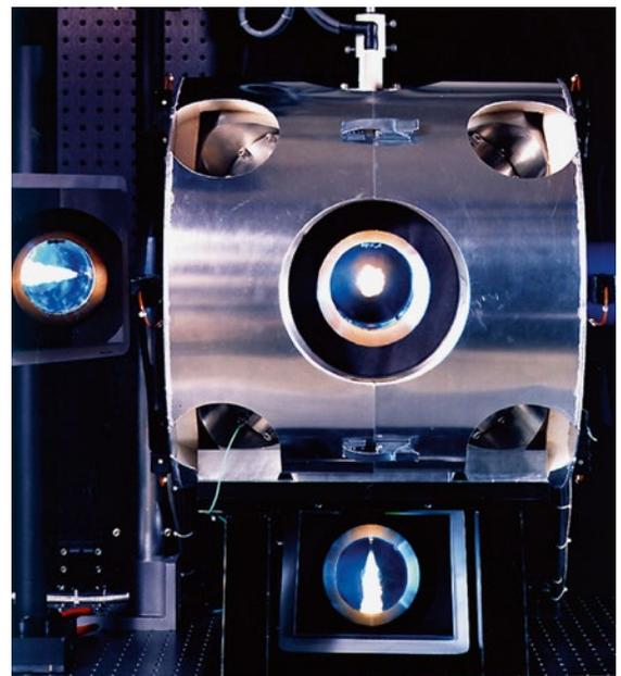
**FIGURE 4** Constant-volume container of the Sandia National Laboratories (SNL) in the USA (© SNL)
