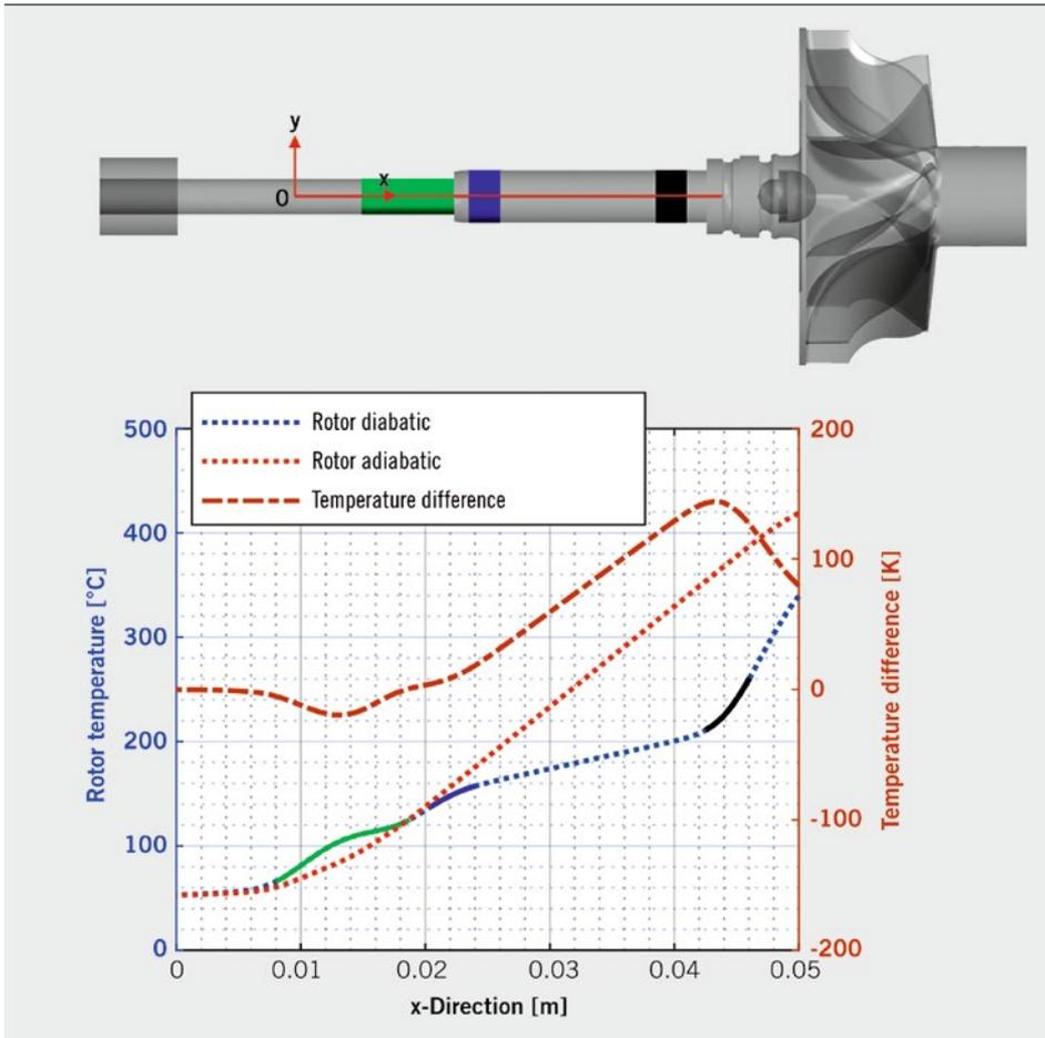
**FIGURE 5** Sketch of the temperature distribution at the rotor (top); rotor temperature analysis under diabatic and adiabatic boundary conditions for OP 2 (bottom) [6] (© LUH | TUC)
