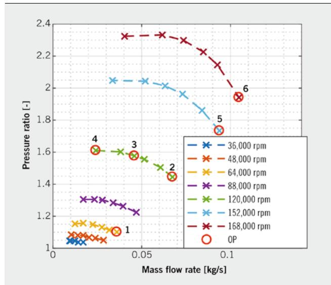
**FIGURE 2** Compressor map of the TC with project-specific OP 1–6 [6] (© LUH | TUC)
