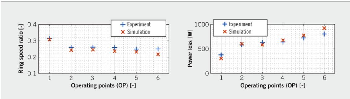
**FIGURE 4** Experimentally and numerically determined ring speed ratio of floating ring to rotor of the compressor-sided journal bearing (left) and the TC power loss (right) for OP 1–6 [6] (© LUH | TUC)
