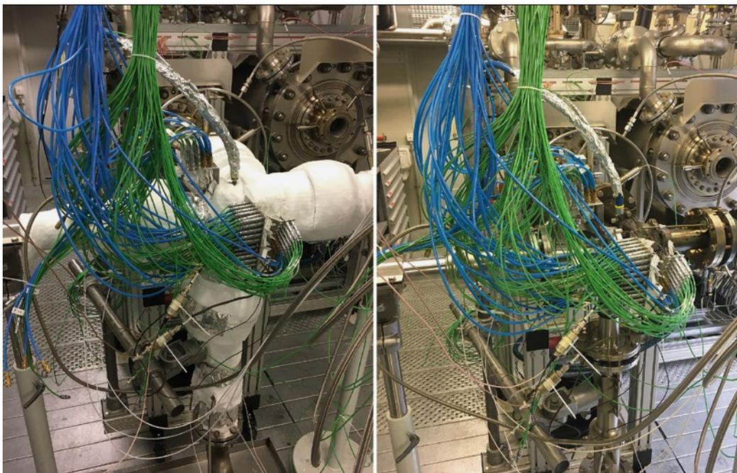
**FIGURE 1** Isolated (left) and non-isolated (right) TC at the TFD test bench (© LUH)
