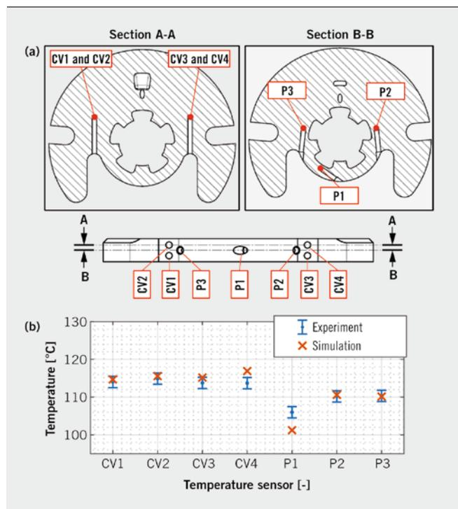
**FIGURE 3** Measuring points of the instrumented thrust bearing (top) and experimentally and numerically determined temperatures for OP 2 (bottom) [6] (© LUH | TUC)
