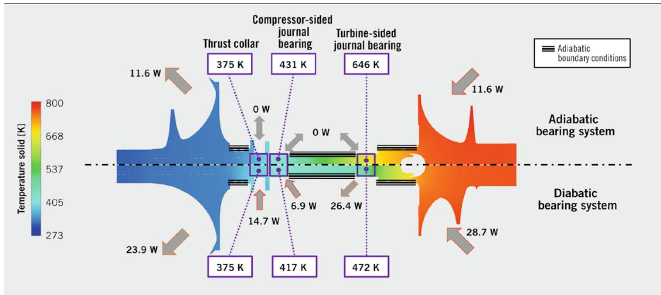
**FIGURE 6** Analysis of heat transfer processes under adiabatic (above the axis) and diabatic boundary conditions (below the axis) for OP 2 (© LUH | TUC)
