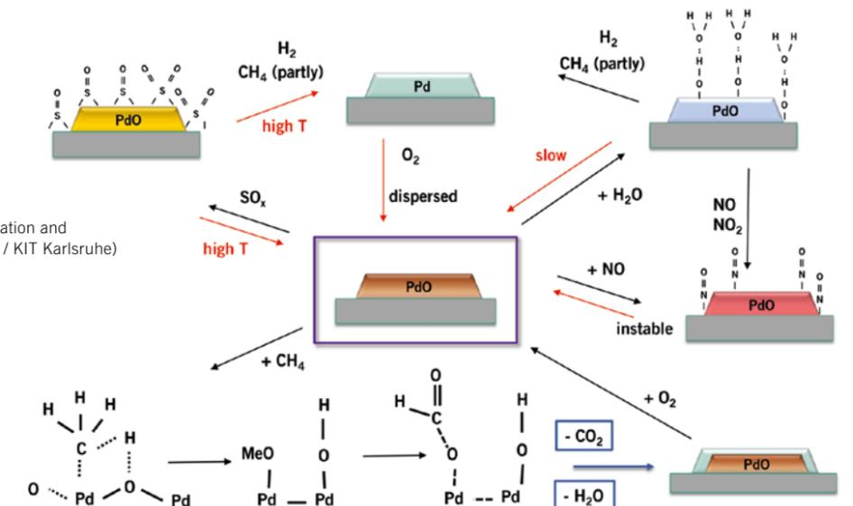
FIGURE 2: Factors that influence the deactivation and reactivation of palladium catalysts (© ITCP / KIT Karlsruhe)
