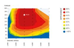
In methanol operation, the new ultimate efficiency engine achieves an efficiency of at least 40% over almost the entire engine characteristic map.
